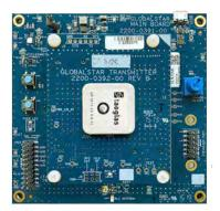
The STX3 Development Kit with Bluetooth<sup>®</sup> Low Energy w(BLE) is an easy way to get set up and send your custom messages over the Globalstar Satellite Network. An accompanying mobile app (compatible with iOS and Android) allows users to issue commands to send accelerometer data, humidity and/ or temperature readings from onboard sensors. Through the mobile app, users can also manually send user-defined custom data via the STX3 module through the Globalstar Satellite Network.
