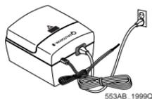
The power supply is selected by the service provider and the installer based on the availability of power at your location. The power supply provides +12 volts to the junction box and RAU.
