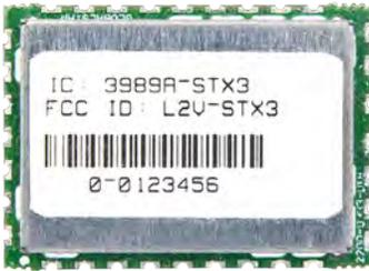
Globalstar offers the STX3 Satellite Transmitter Unit to help customers design and build compact and efficient communications devices. Using the Globalstar Satellite Network, the STX3 allows information to be transmitted from areas well beyond the reach of reliable cellular coverage around the globe.
