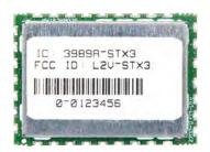
Globalstar offers the STX3 Satellite Transmitter Unit to help customers design and build compact and efficient communications devices. Using the Globalstar Satellite Network, the STX3 allows information to be transmitted from areas well beyond the reach of reliable cellular coverage around the globe.
