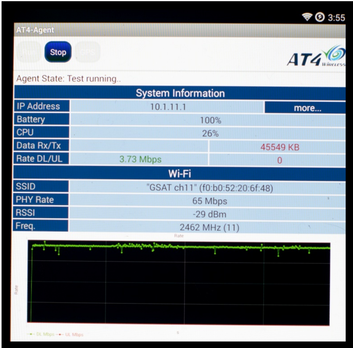
Photograph 2: Photograph of Nexus tablet client devices showing display of measurement conditions during Bluetooth SIG demonstration. 3.73 Mbps download to clients.
