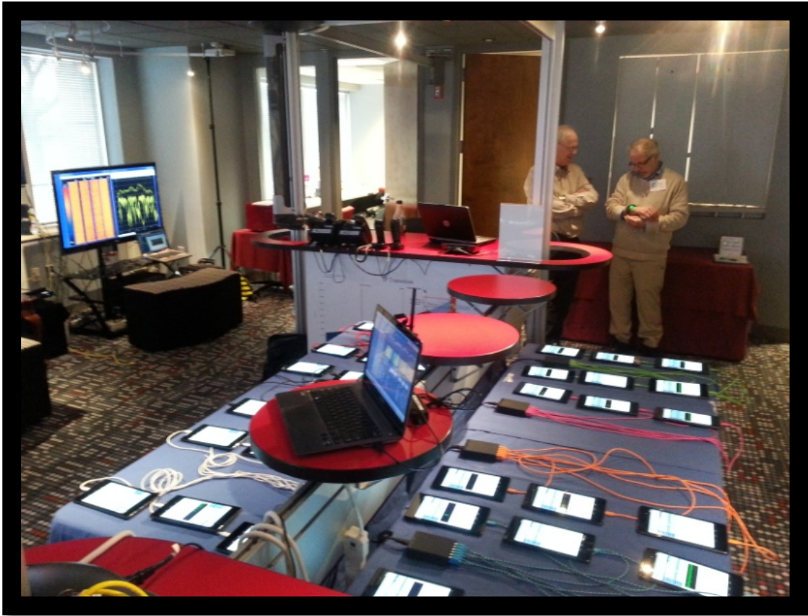
Photograph 1: Photograph of client devices in FCC TEC. One access point visible on pole at upper left. Other access points located at corners of the room with clear visibility to client devices.
