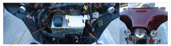
SPOT Trace mounted under the fiberglass fairing of a motorcycle using the included Velcro strip and mounting bracket.
