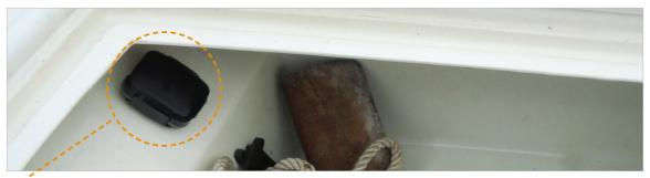
SPOT Trace mounted inside a fiberglass compartment of a boat using the included Velcro strip and mounting bracket. Notice the unit is angled toward the sky for optimal performance.
